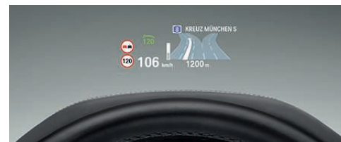
□ The full-colour BMW Head-Up Display 3 projects relevant driving information directly into the driver's line of sight, allowing the driver to concentrate more closely on the road ahead. The display includes information such as the current speed, navigation directions, Speed Limit Info incl. no-overtaking indicator, along with telephone and entertainment lists.
