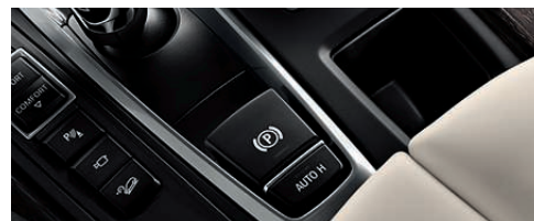
■ Parking brake with auto-hold function can be conveniently activated via a button in the centre console. The brake is released once the accelerator is depressed. The auto-hold function assists the driver in stop-start traffic, or during hill starts, by preventing the car from rolling forwards or backwards when at a standstill.
