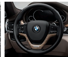
□ BMW Individual leather steering wheel in the sport leather steering wheel design with wooden inlays to match the respective BMW Individual interior trim.
